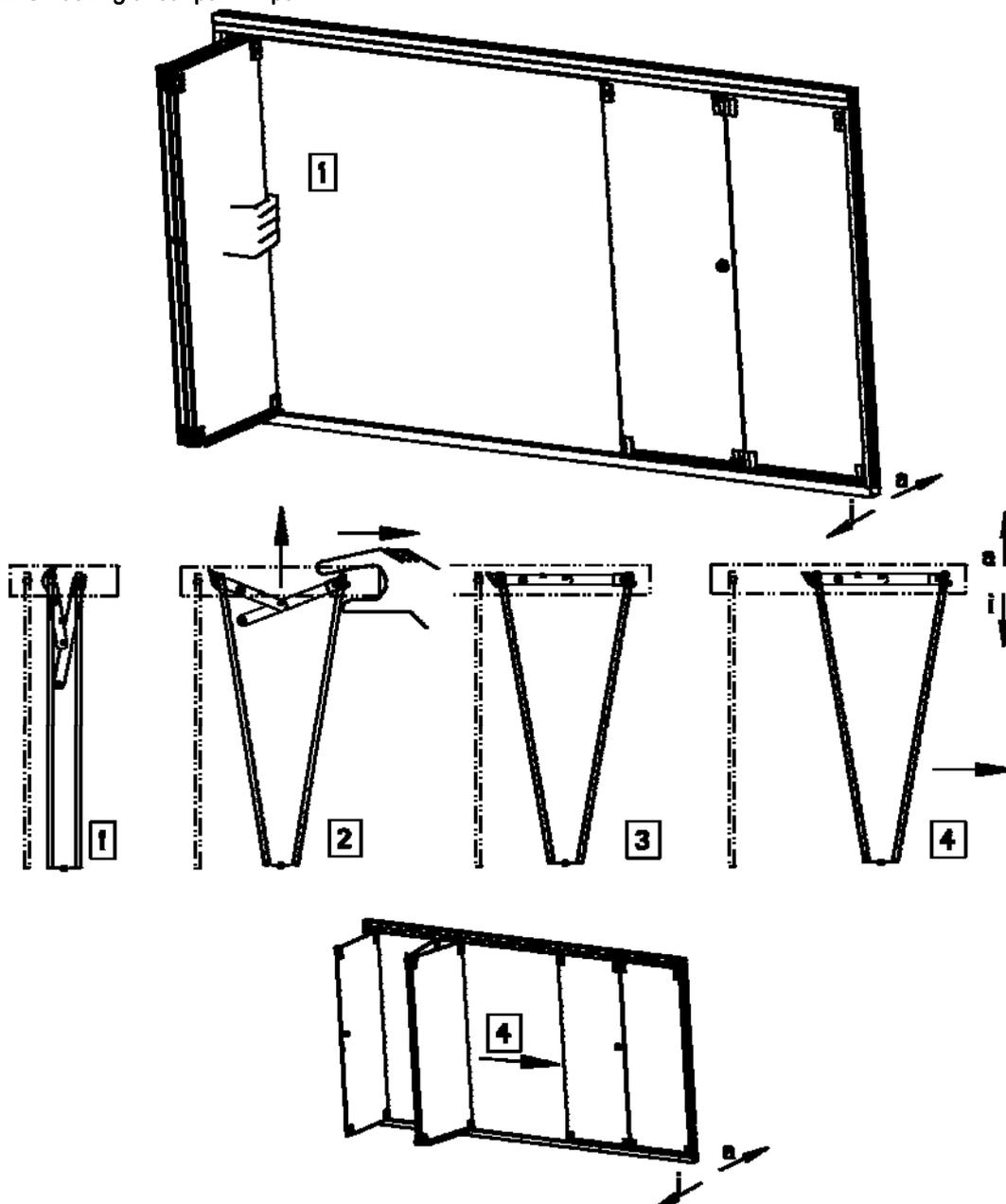
**i** If the opening limiter has not engaged, pull the leafs apart while pulling the opening limiter straight using your hand or foot, as shown here.
