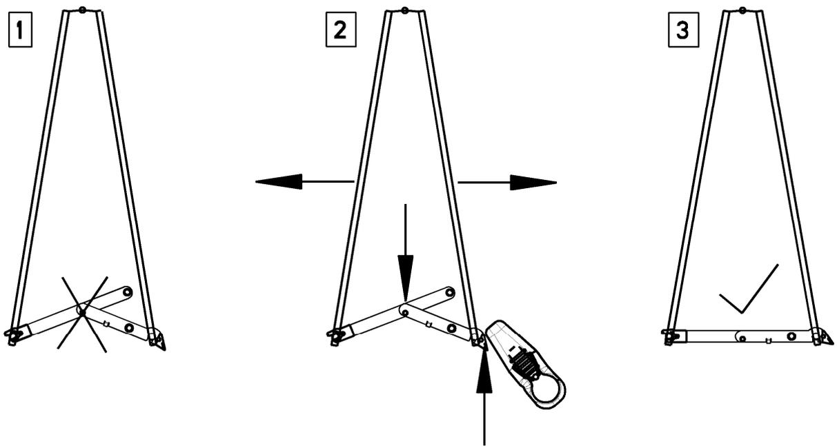
6.8.2 Releasing the leaves from the V-position, locking them into a closed position
